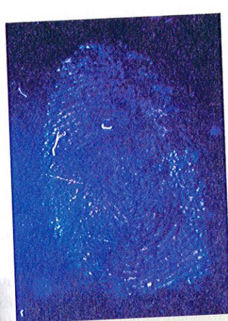
Figure 6.9G Latent fingerprint visualized by Super Glue fuming and washing with laser dye Ardrox to produce a fluorescent print.
